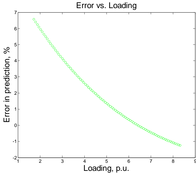
Figure 4.11 Error for the two bus system using the proposed method
