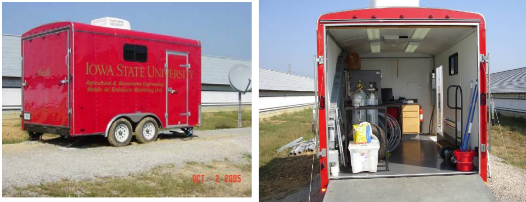
Figure 1. Environmentally-controlled Mobile Air Emissions Monitoring Units (MAEMU).
