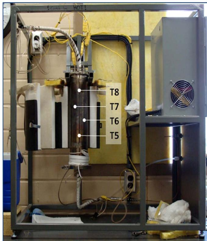
Figure 1. Position of four thermocouples utilized for controlling the temperature inside the reactor
