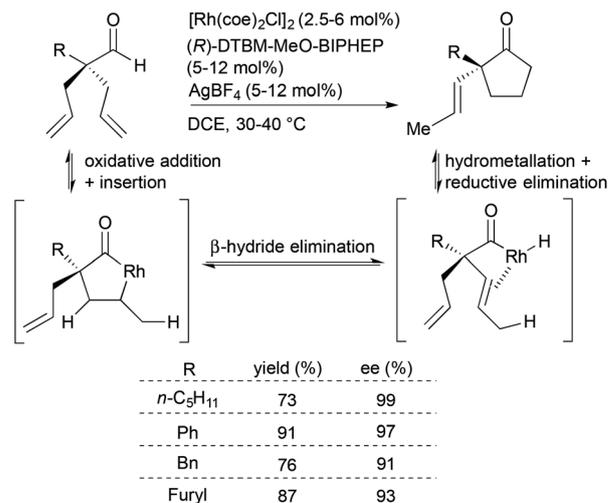
**Scheme 3** Desymmetrization of  $\alpha$ -quaternary centers by isomerization–hydroacylation.
