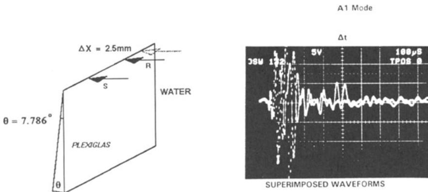
Fig. 7. Measurement of A1 mode phase velocity for immersed small-angle ( $\theta = 7.786^\circ$ ) Plexiglas wedge in water. A 2.50 mm displacement produces  $45.0\ \mu\text{s}$  time delay. Photograph showing superposition of waveforms detected at two ranges  $X = 2.1911\ \text{cm}$  and  $2.441\ \text{cm}$ .
