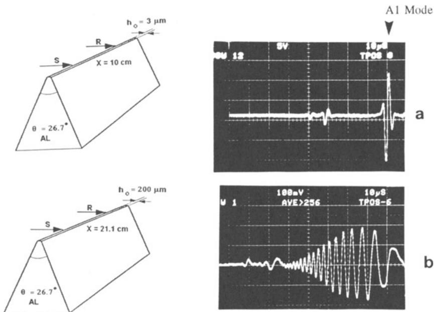
Fig. 1. Experimental setup configuration and waveform of antisymmetric wedge waves along apex of aluminum wedge with apex angle  $\Theta = 26.7^\circ$ . Top: sharp apex ( $h_0 = 3 \mu\text{m}$ ). Bottom: truncated wedge ( $h_0 = 200 \mu\text{m}$ ).
