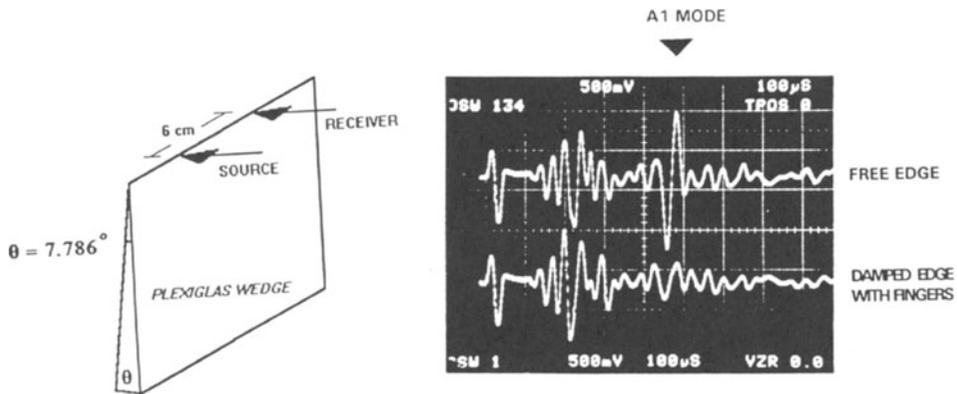
Fig. 5. Extremely slow flexural edge waves observed propagating along edge of free Plexiglas wedge with small apex angle  $\theta = 7.786^\circ$ . Top: arrow pointing to A1 mode. Bottom: wedge edge damped with finger tips to attenuate the A1 mode.
