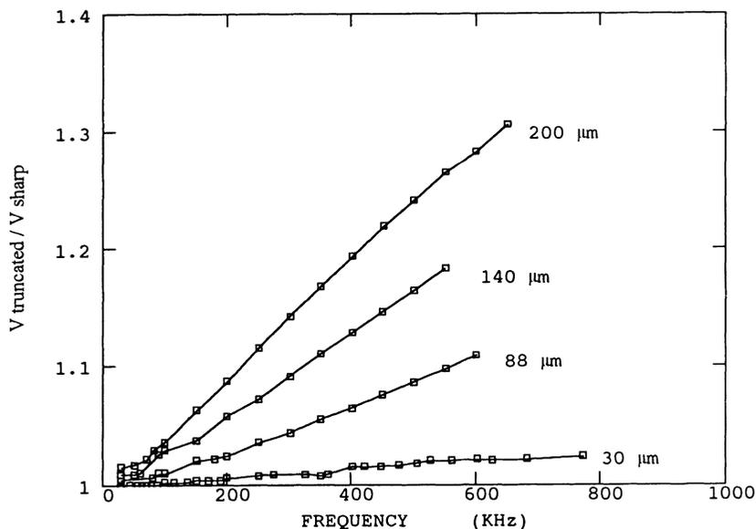
Fig. 2. Dispersion of slowest antisymmetric edge wave from truncated aluminum wedge for different values of  $h_0$  (30, 88, 140, and  $200 \mu\text{m}$ ). Ratio of A1 wedge mode (phase velocity of truncated wedge) / (phase velocity of sharp wedge) plotted as a function of frequency in KHz.
