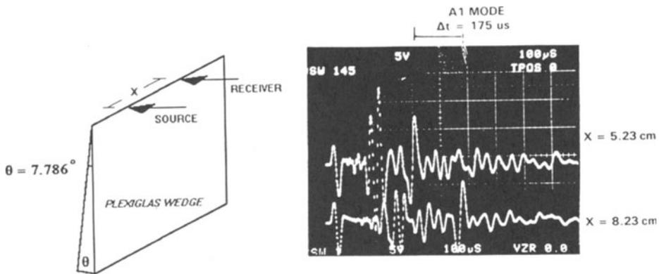
Fig. 6. Measurement of A1 mode phase velocity for small-angle ( $\theta = 7.786^\circ$ ) Plexiglas wedge in air. A 3.00 cm displacement introduces a  $175\ \mu\text{s}$  time delay.
