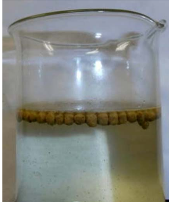
Picture 1. All extrudates from diet 1 (20% DDGS), diet 2 (40% DDGS), diet 3 (20% HP-DDG), and diet 4 (40% HP-DDG) floated for more than 25 min.
