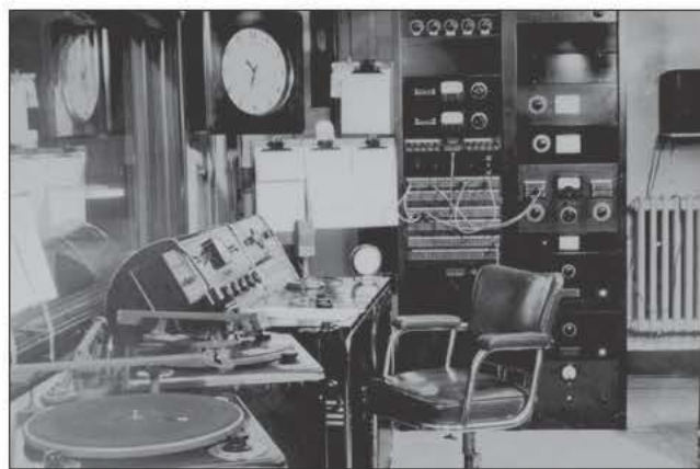
Figure 1: The Control Room of Omaha radio station KFAB, c. 1935, shows two electrical transcription disc machines in the lower left foreground: the nearest is a player, and behind it is an instantaneous disc recorder. Courtesy Nebraska State Historical Society.
