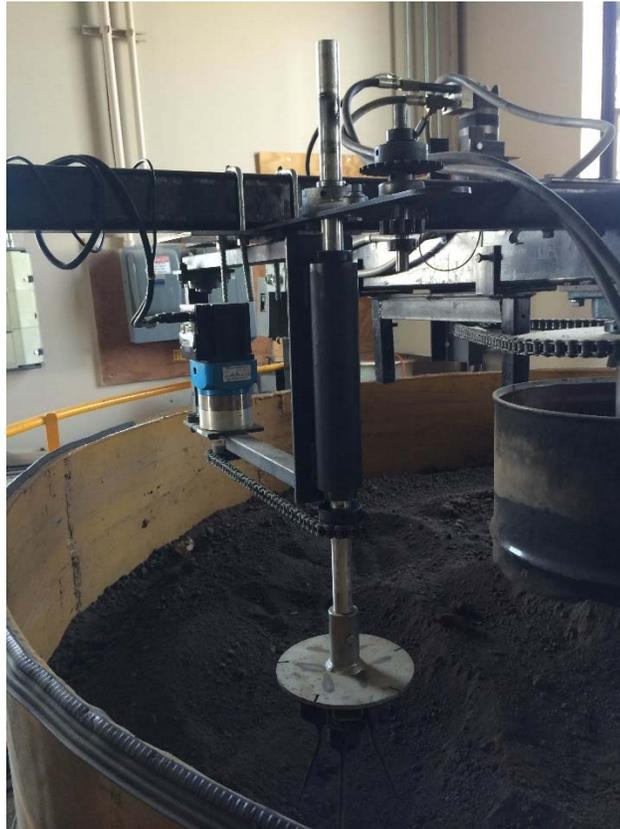
Figure 2: Prototype mechanical weed control in a soil bin
