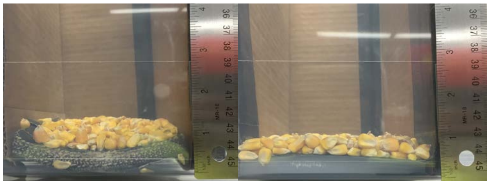
Figure 5: Grain pile loading on paddle sets 1 and 3 for 5 kg s -1 mass flow rate, respectively
