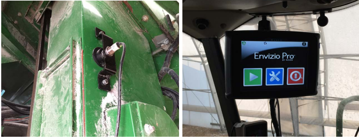
Figure 2: SmartYield Pro yield monitor beam-based volumetric flow sensor and display, respectively
