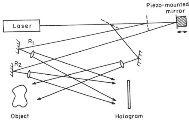
Figure 2 - Arrangement for quasi-heterodyne holographic interferometry.
