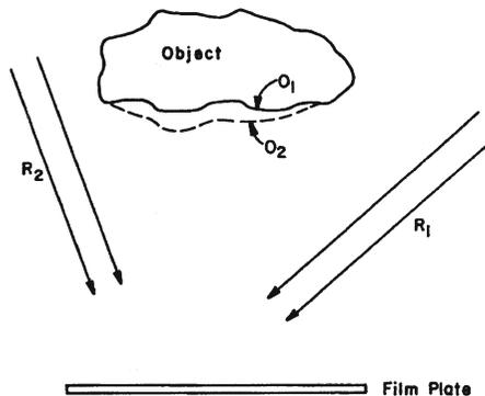
Figure 1 - A setup for recording two-reference-beam holograms.
