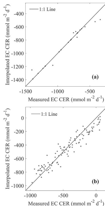
Fig. 2. Comparisons of the measured daily eddy covariance  $\text{CO}_2$  exchange rate (EC CER) and the predicted daily EC CER for (a) corn, 2013, and (b) soybean, 2014.
