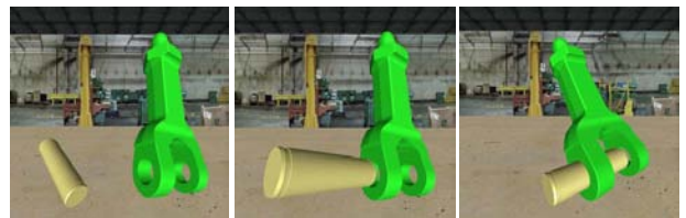
Figure 4: Assemble of a pin-in-a-hole using automatic geometric constraints [26]
