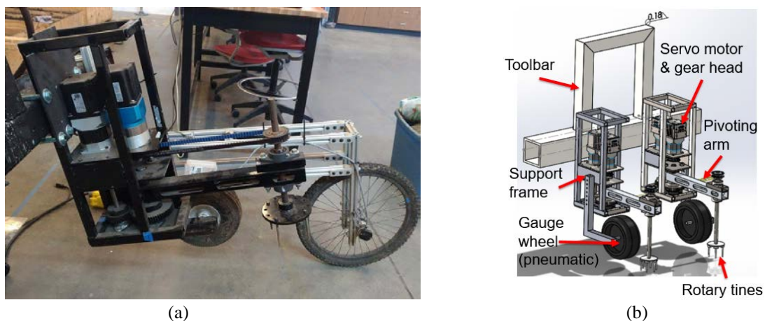
Figure 1. Automatic weeder used in vibrations tests mounted in a tractor (a) and the weeder mechanism with details of its components (b).
