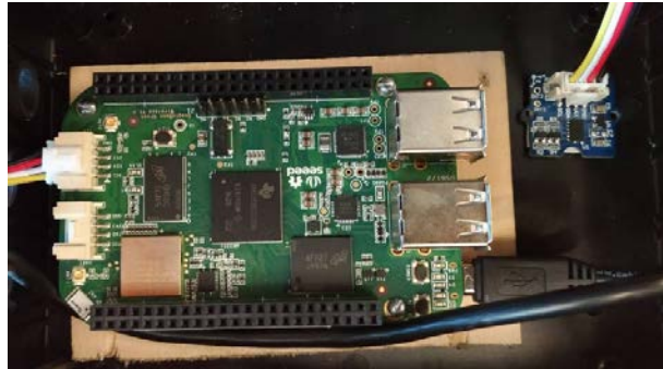
Figure 2. Single board computer Beaglebone Green Wireless® and the ADXL345 digital MEMS accelerometer used on vibrations tests.
