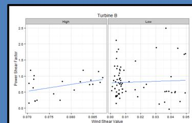
FIG 2: Turbine power factor as a function of wind shear for turbine B.
