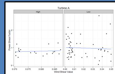
FIG 1: Turbine power factor as a function of wind shear for turbine A.
