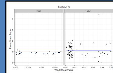
FIG 4: Turbine power factor as a function of wind shear for turbine D.
