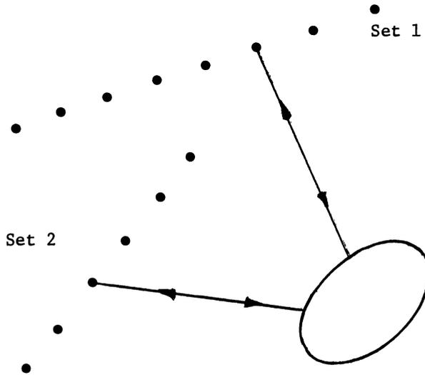
Fig. 1. Configuration of source-receiver positions and crack.
