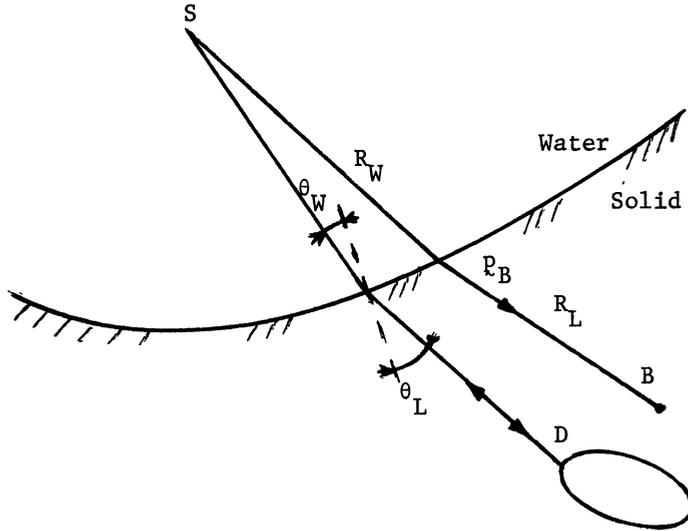
Fig. 2. Water-bath configuration for pulse-echo measurements; S-transducer, B-base point: D-flash point.
