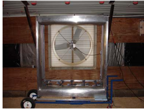
Fan calibration by FANS unit
