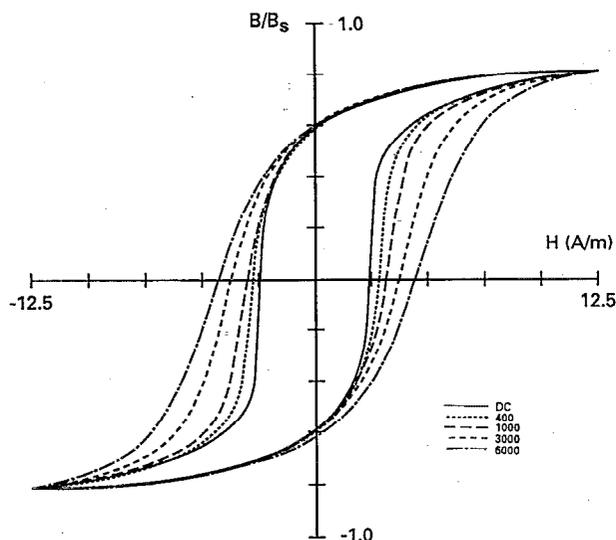
FIG. 2. Modeled hysteresis curves of Permalloy 80 at dc, 400, 1000, 3000, and 6000 Hz calculated by incorporating effects of classical eddy current power losses into the hysteresis equation.
