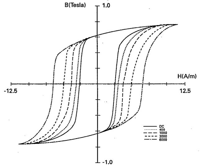
FIG. 1. Measured hysteresis curves of Permalloy 80 at dc, 400, 1000, 3000, and 6000 Hz (see Ref. 15).
