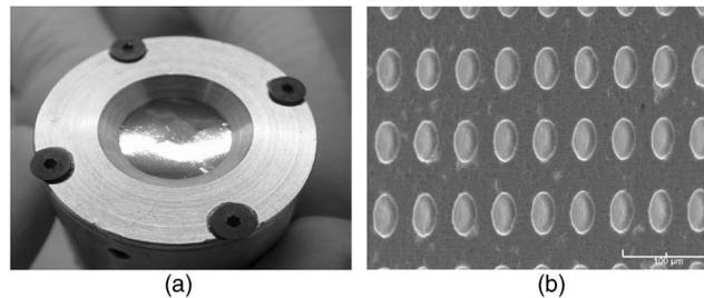
Fig. 1. (a) A photograph of a 5 mm radius, 25.4 mm focal length spherically focused capacitive micromachined air-coupled ultrasonic transducer. A white line on a 6  $\mu\text{m}$  Mylar/Al film is the reflection of a light source. (b) A SEM image of a flexible copper/polyimide backplate.
