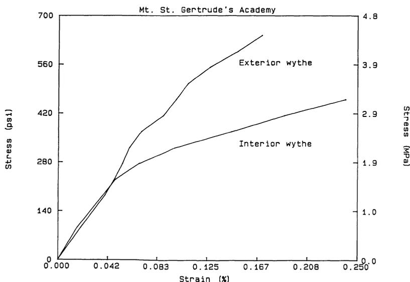
Figure 4. Example Stress-Strain Curves Obtained from Flatjack Tests on an Existing Masonry Structure.
