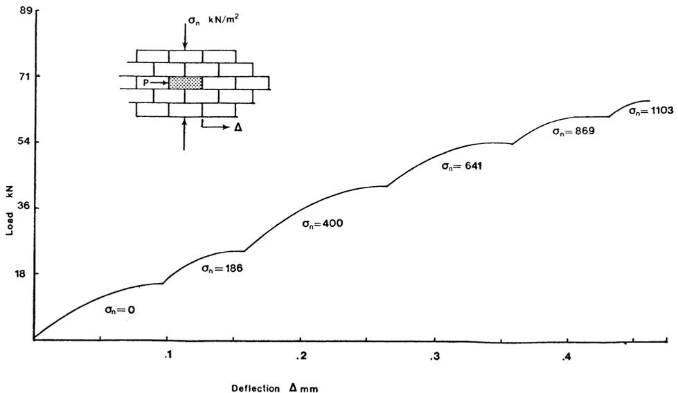
Figure 5. Typical Results from a Modified In-Place Shear Test.
