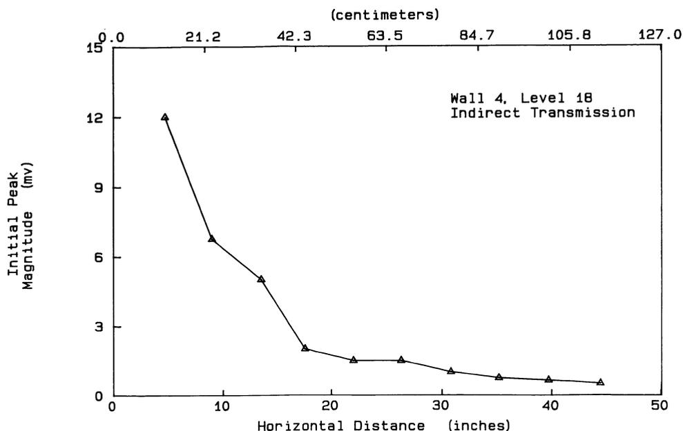
Figure 2. Ultrasonic Pulse Signal Attenuation.
