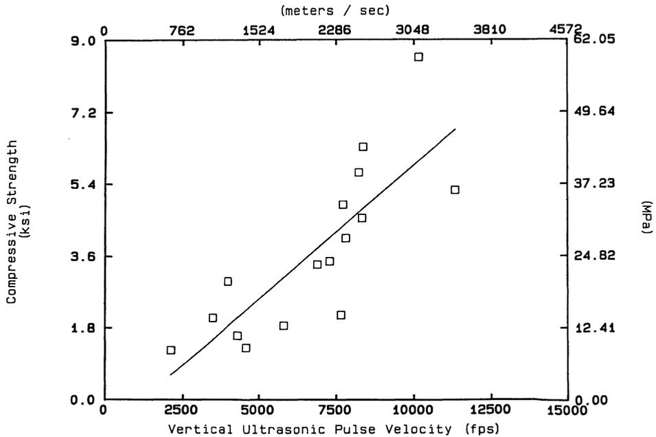
Figure 1. Correlation of Ultrasonic Pulse Velocity with Masonry Prism Compressive Strength.
