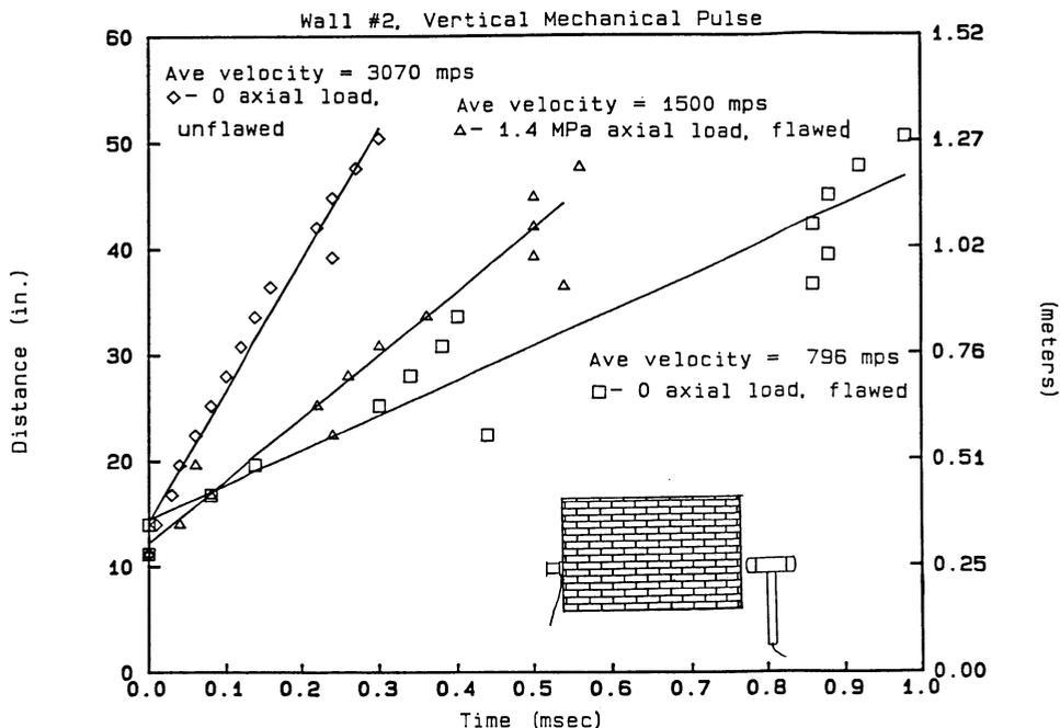
Figure 3. The Effect of Flaws and Compressive Stress on Mechanical Pulse Velocity.
