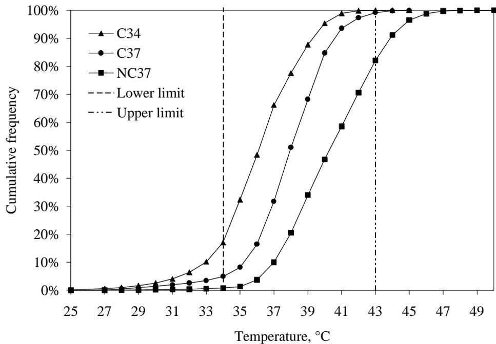
**Figure 7. Frequency distribution of mat temperature measured by thermocouples. °F = °C × 1.8 + 32.**
