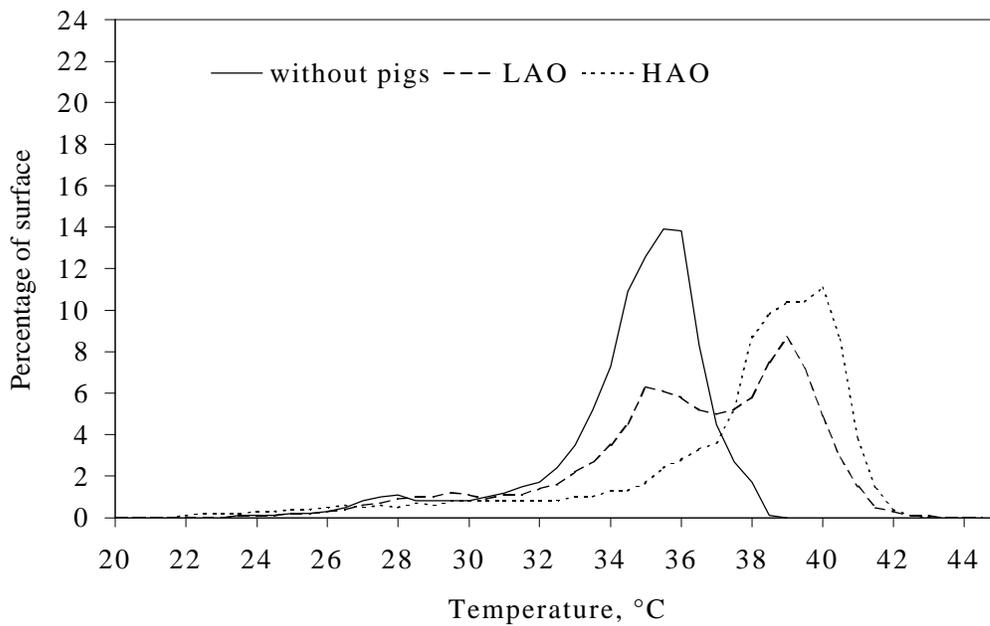
**Figure 5. Surface temperature distribution of heat mat without temperature feedback control and at set temperature of 37°C (99°F) (NC37). °F = °C × 1.8 + 32.**
