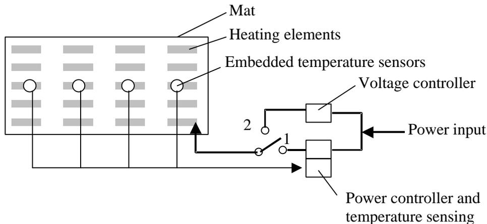
**Figure 1. Schematic representation of heat mat layout and power input control.**
