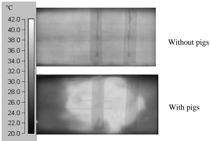
Figure 2. Comparison of mat temperature distribution without vs. with pigs.
