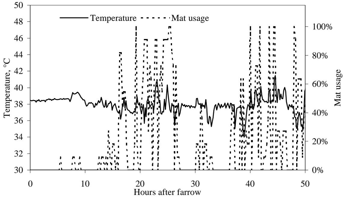
**Figure 6. Typical pattern of mat temperature variation with time and mat use by pigs (Test C37) (Note: A heat lamp was available in the back of the crate for the first 48 h).**
