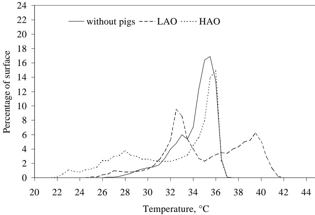
**Figure 4. Surface temperature distribution of heat mat with temperature feedback control and at set temperature of 37°C (99°F) (C37). °F = °C × 1.8 + 32.**
