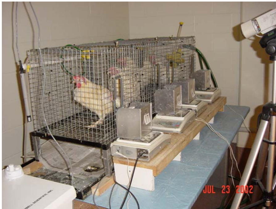
Figure 1. Photographical view of the testing room showing four individual cages with a feeder attached to an electronic balance, a temperature/relative humidity probe, and monitoring video cameras.
