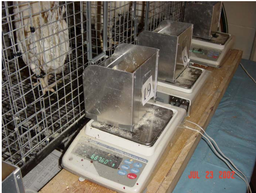
Figure 2. GX2000 electronic balances with analog output used in the feeding behavior study.
