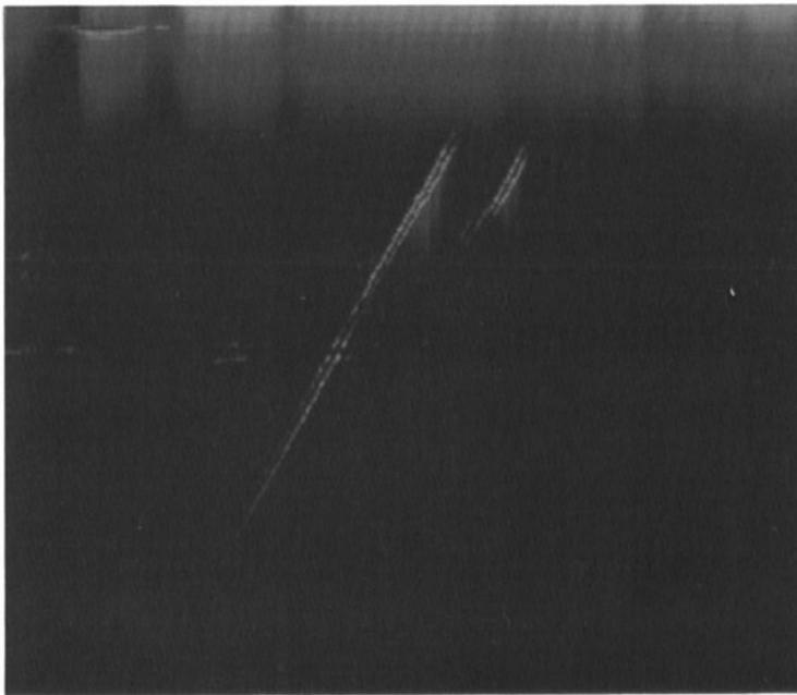
Fig. 1. Image formed by a SLIC-50 transducer before processing
