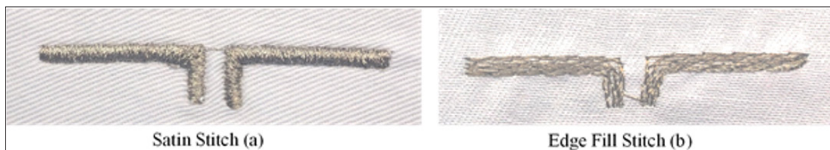
Figure 7: Physical samples of dipole antenna stitched through machine embroidery.
