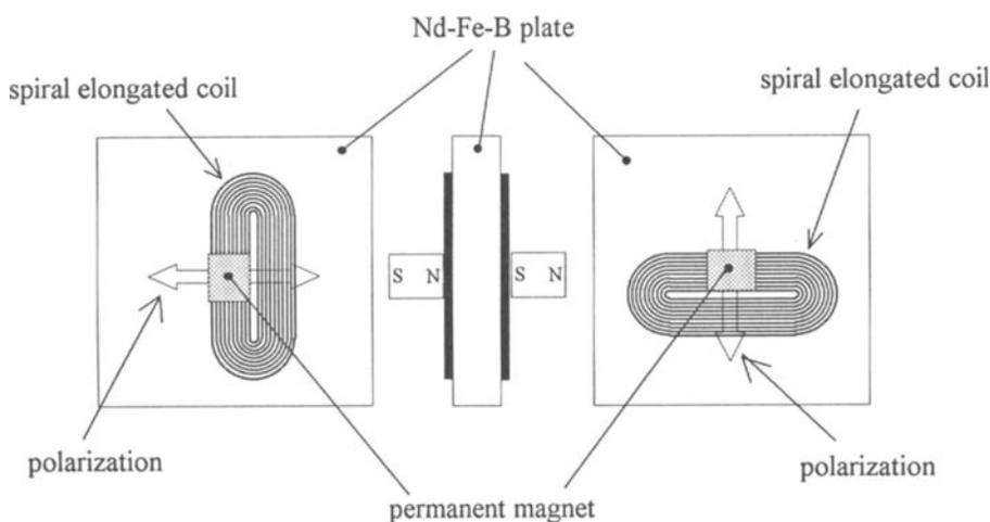
Figure.1 Measurement configuration of the two shear wave EMATs.
