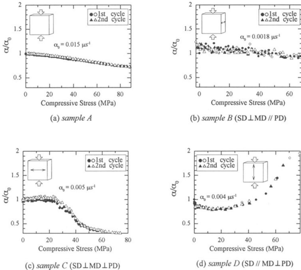
Figure 5. The attenuation response of the shear wave polarized in the stress direction.  $\alpha_0$  is the original attenuation coefficient. Solid and open marks indicate the data at loading and unloading sequences, respectively.
