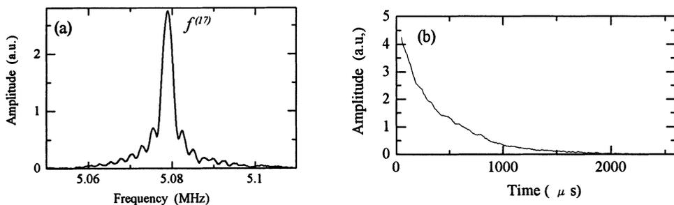
Figure.3 (a) Resonant spectrum and (b) ringdown curve observed in *sample A*.
