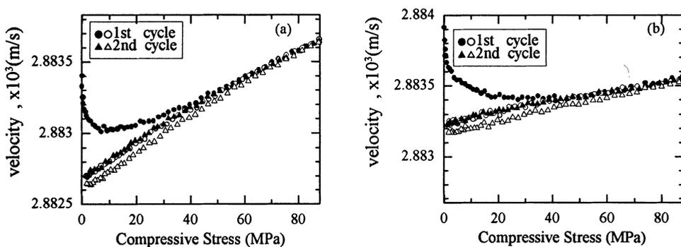
Figure 4. The velocity response in *sample A*. (a) Polarization in the stress direction and (b) polarization normal to the stress. Solid and open marks denote the data at loading and unloading sequences, respectively.
