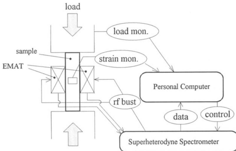
Figure.2 Measurement setup with two EMATs and superheterodyne spectrometer.
