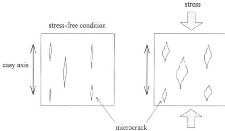
Figure 6. Model for the microcrack alignment to the easy axis.
