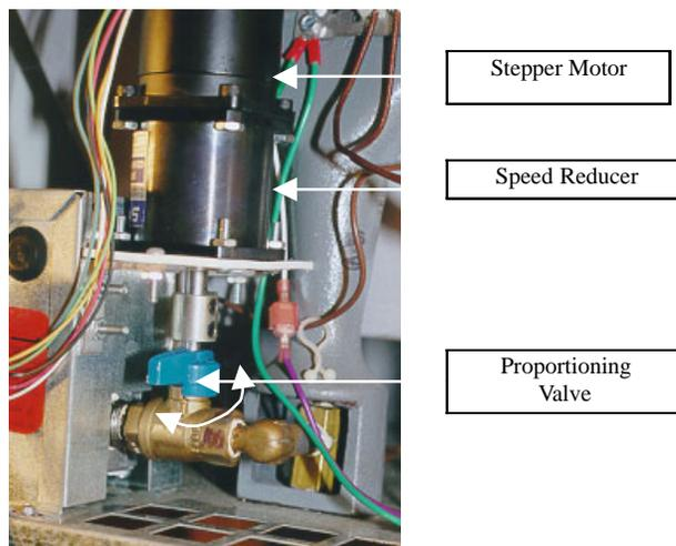
**Figure 2.** Manual proportioning valve as a standard feature of the heater with modifications attached for automated variable control (AVC).
