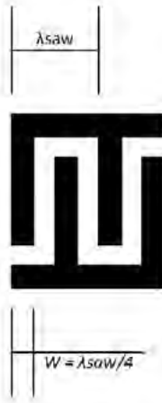
Figure 5. IDT finger width and inter-IDT spacing relationships
