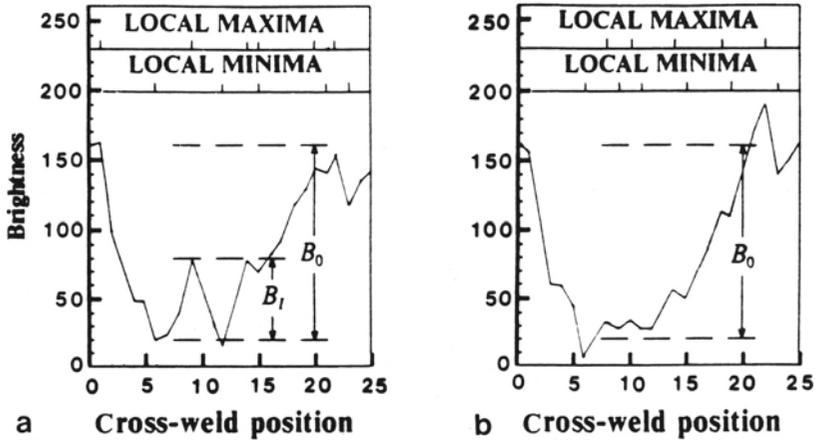
Fig. 3 Brightness profile across image of weld (a) incomplete and (b) complete welds.  $B_0$  is difference in brightness levels between base metal and weld reinforcement.  $B_1$  is brightness difference between brightness levels of complete and incomplete weld.
