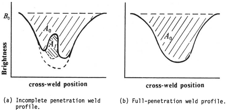
Fig. 4 Schematic showing area of profiles taken into account in second criterion on weld penetration.
