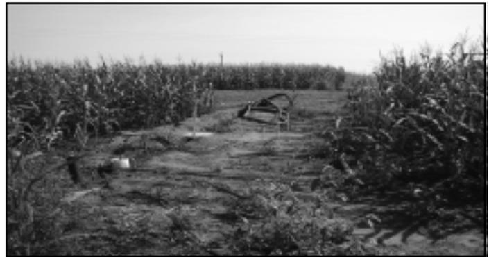
Looking down-slope at trench and solution addition point on left, three sampling wells in center.
