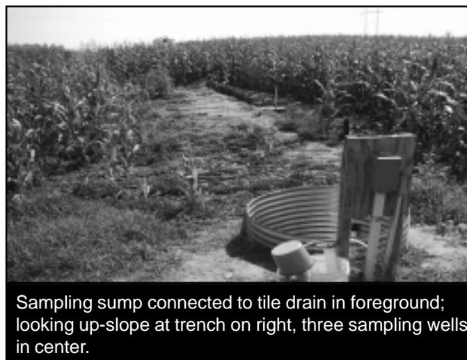
Sampling sump connected to tile drain in foreground; looking up-slope at trench on right, three sampling wells in center.
