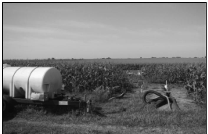
Source tank for solution of P and tracer (Br) on left; trench on right, three sampling wells in center, and sampling sump connected to tile drain at far end.
