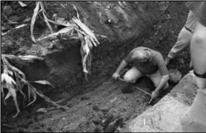
Horizontal sampling of the subsoil in the face of a trench following P addition.
