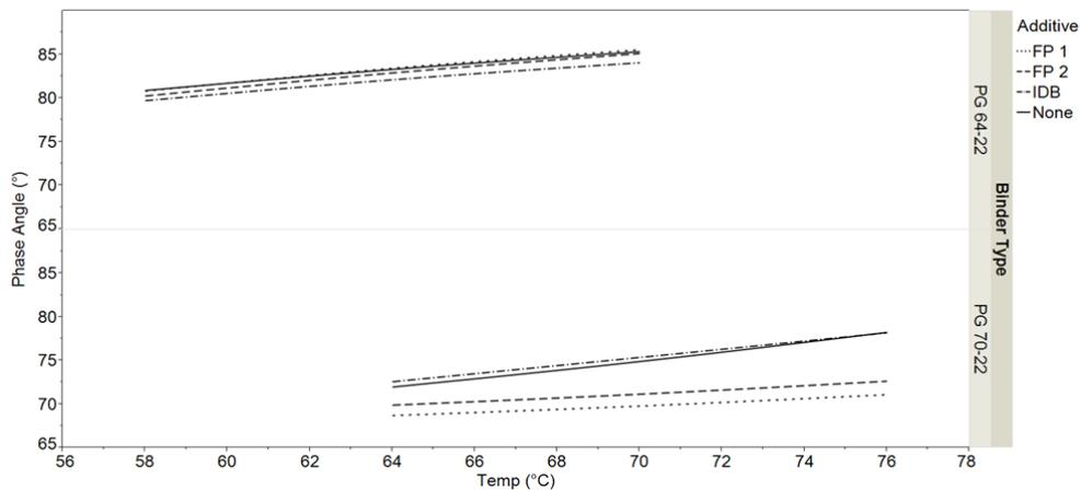
Fig. 5: Comparison of Average Phase Angle results
