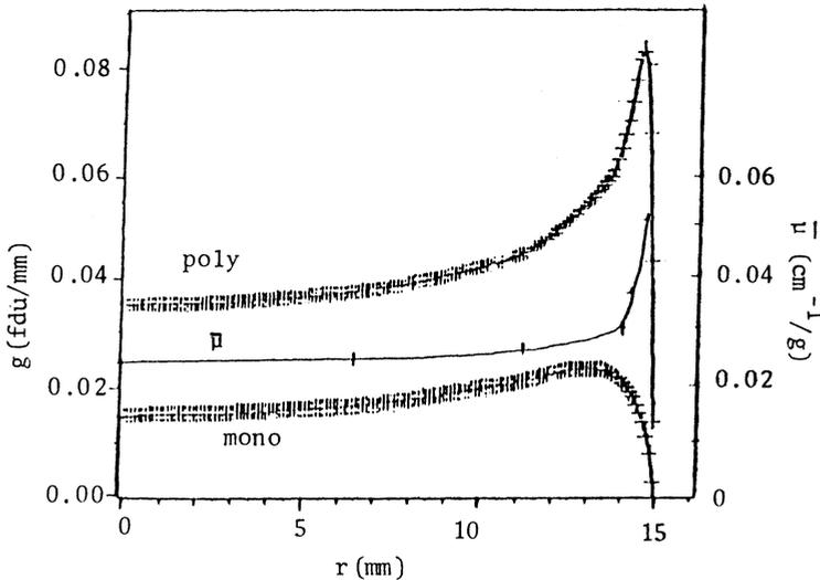
Fig. 3 Reconstructed profiles from radiographs of an Al cylinder (1.46 cm radius) with 130 kV x-rays (poly) and Cs-137 gamma rays (mono). Average attenuation coefficient for 130 kV is indicated by  $\bar{\mu}$ .
