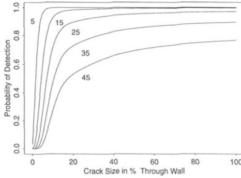
Figure 4. PODcurves for different detection threshold levels.
