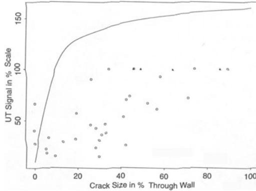
Figure 2. UT measurements and theoretical model prediction.
