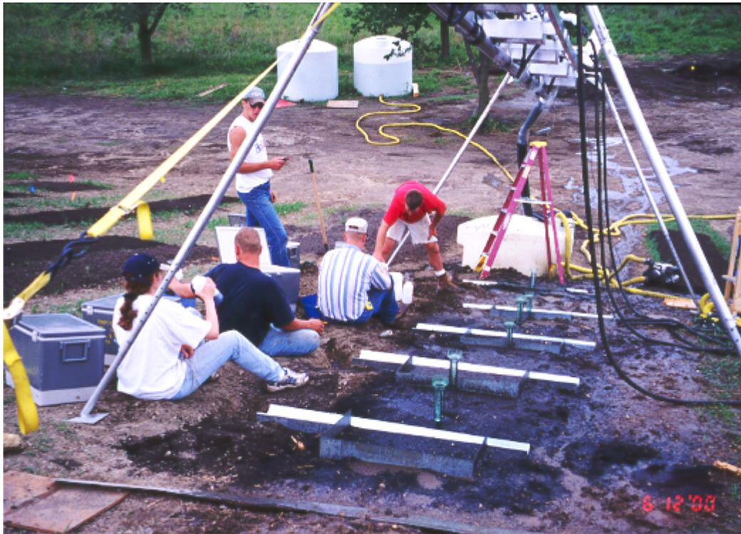
Figure 1. Rainfall simulator and test plot setup during interrill runoff sampling.
