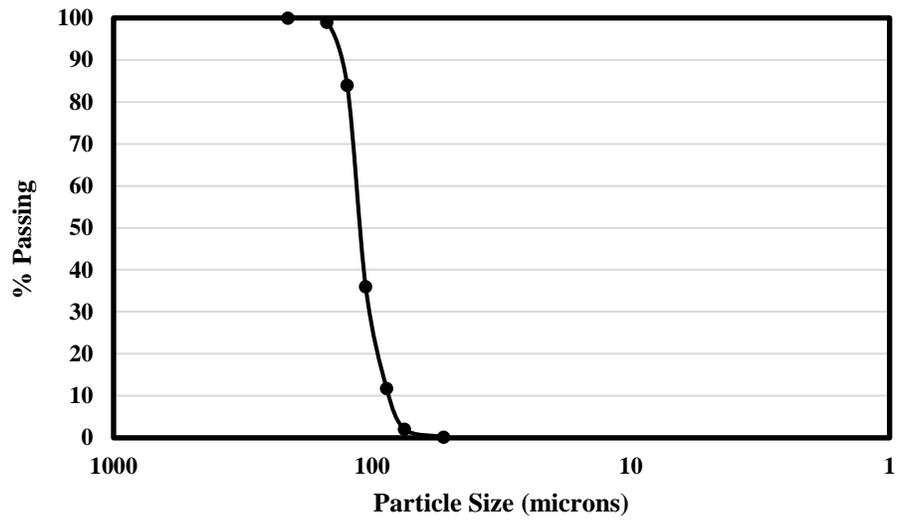
**Fig. 1.** Particle size distribution of OK-110 silica sand.
