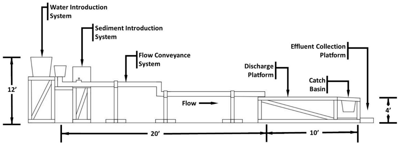
**Fig. 2.** Schematic of CBI testing apparatus.
