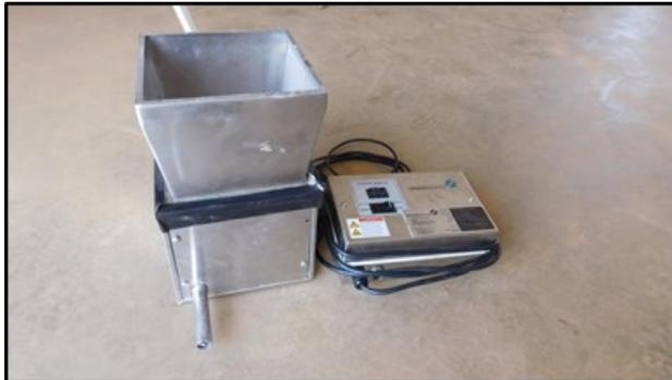
(c) Schenck Process Model 106M Material Feeder
