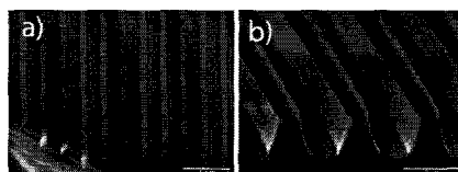
Figure 7.11 (a) After Ar plasma etching the top Au layer deposited on the polymer, and the polymer template were etched away, leaving single sidewalls on the substrate. (b) Etched top of the gold having double sidewalls with Ar ion milling. The polymer templates (PU) were partially etched and remained between the metals.
