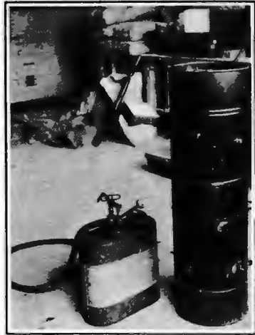
Fig. 9. Oil tank and spray pump for oiling forms.
