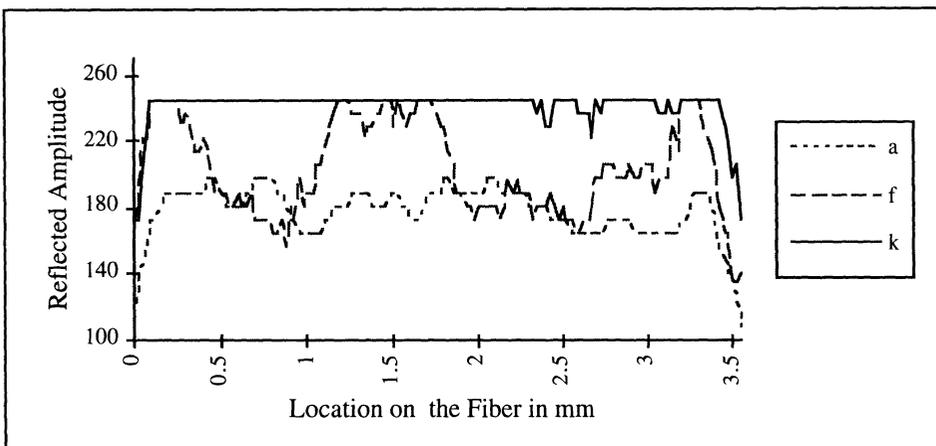
Figure 3 Ultrasonic Reflectivity from the Fiber-Matrix Interface at Various Locations for Selected Stages of Loading of the Test Specimen (indicated by a, f, and k in Figure 2).
