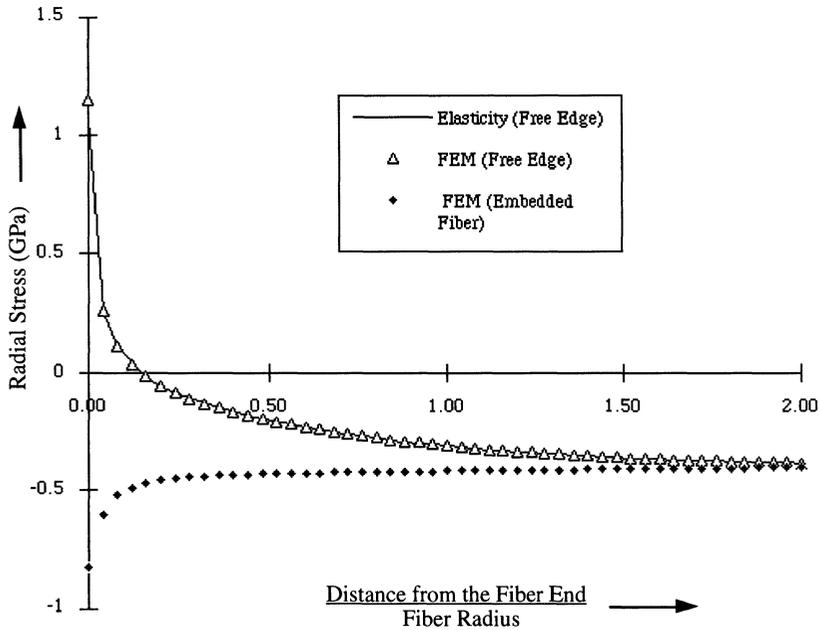
Figure 5 Interfacial radial stress distributions near the fiber tip.
