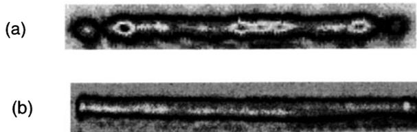
Figure 4 Ultrasonic shear wave images of (a) fiber with free edge, and (b) completely embedded fiber.
