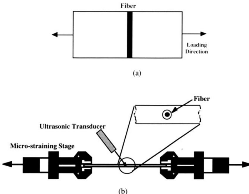
Figure 1 (a) Experimental Configuration Showing Transverse Orientation of the Fiber in a Sample and the Direction of Loading. (b) Configuration of the Micro-Straining Stage for Ultrasonic In-Situ Imaging Arrangement.
