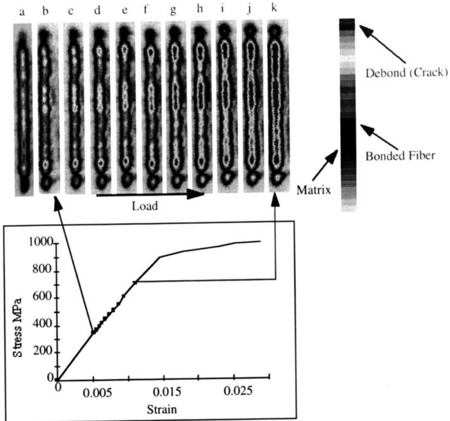
Figure 2 In-situ Ultrasonic Imaging of an Embedded Fiber During Various Stages of Loading.
