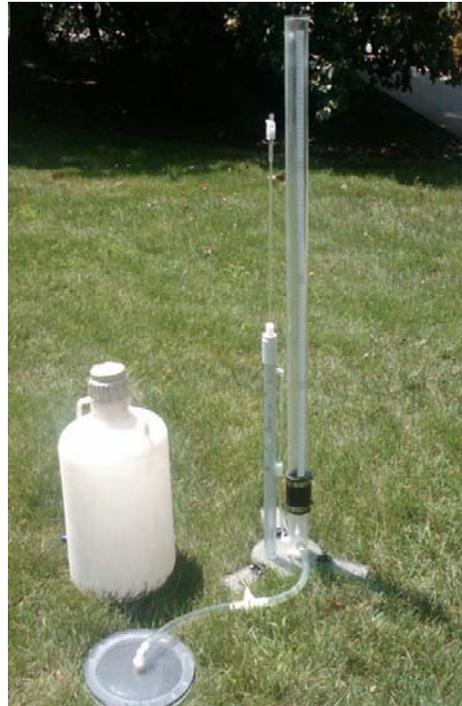
Figure 2. Schematic of Tension Infiltrometer; a)Rubber stopper, b)Water level, c)Tygon tubing for pressure transducer, not used in 2010, d)Reservoir, e)Infiltration disc, f)Base, g)Air bubbling tube, h)Air bubble tower, i) Water level, j) Air entry tube, and k) hose clamp and Picture of actual tension infiltrrometer used.
