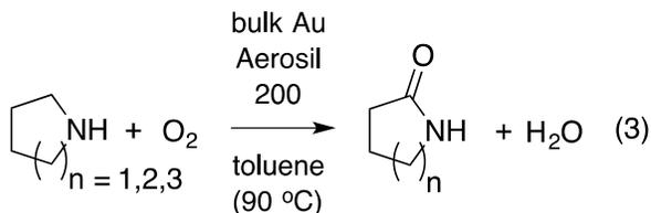
efficiency of Au when supported on high surface area metal oxides [38, 39], including CeO<sub>2</sub> [32], prompted us to explore the activity of Au/CeO<sub>2</sub> in the oxidation of cyclic amines to lactams. We report herein that Au/CeO<sub>2</sub> efficiently catalyzes the oxidation of both cyclic secondary and N-methyl cyclic tertiary amines to the corresponding lactams.
