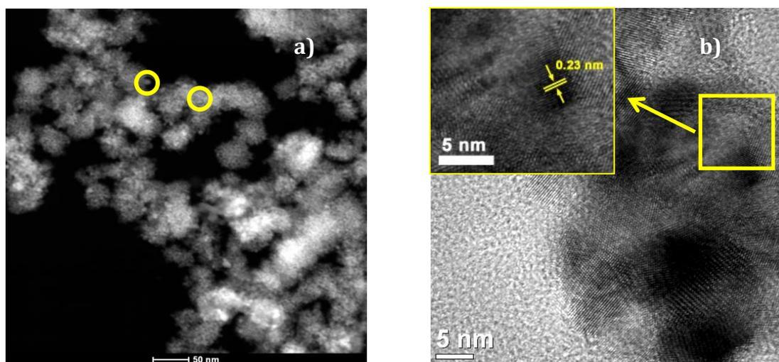
**Figure 1.** (a) Scanning transmission electron microscopy (STEM) image of the unused 5.4 wt% Au/CeO<sub>2</sub> catalyst. Circles indicate representative Au nanoparticles. (b) High-resolution transmission electron microscopy (HR-TEM) image showing the presence of Au particles on the surface of CeO<sub>2</sub> for the unused 5.4 wt% Au/CeO<sub>2</sub> catalyst.
