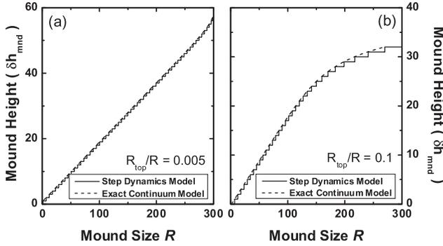
FIG. 4. Comparison of the selected mound shapes obtained from step dynamics model and the exact continuum Eq. (9).  $P_+ = 0.55$ ,  $c = 1/2$ ,  $b = 1$ , and  $R = 300$ . (a)  $R_{\text{top}}/R = 0.005$ ; (b)  $R_{\text{top}}/R = 0.1$ .
