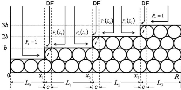
FIG. 1. Schematic of step dynamics model showing deposition, DF, and surface diffusion processes.  $x = 0$  ( $R$ ) denotes the mound valley (peak),  $x_i$  the position of step  $i$ , and  $L_i$  the width of terrace  $i$ .  $P_+$  ( $P_-$ ) gives the probability of diffusing to ascending (descending) steps. “Step edge regions” have width  $c$ .
