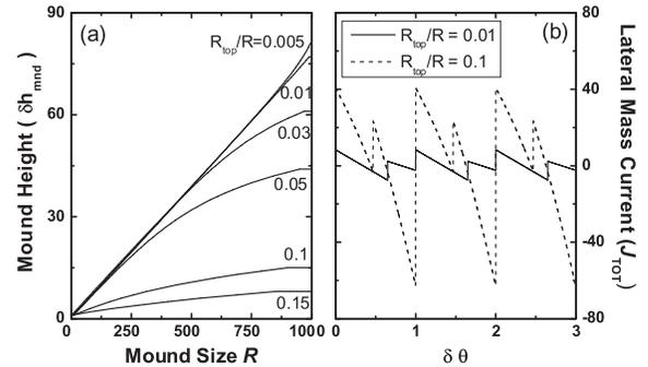
FIG. 2. (a) Selected mound shapes for various choices of  $R_{\text{top}}$  for nucleation; (b) periodic variation of the total mass current,  $J_{\text{TOT}}$ , with coverage increment,  $\delta\theta$ , for different  $R_{\text{top}}$ .  $\delta\theta = 0$  corresponds to top layer nucleation. Here  $P_+ = 0.52$ ,  $c = 1/2$ ,  $b = 1$ , and  $R = 1000$ .
