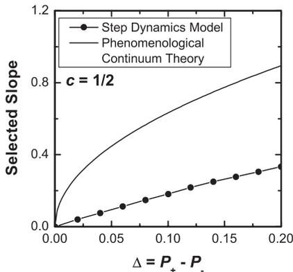
FIG. 3. Comparison of the behavior of the selected slope with  $\Delta$  obtained from step dynamics model and the phenomenological continuum theory for  $b = 1$ .
