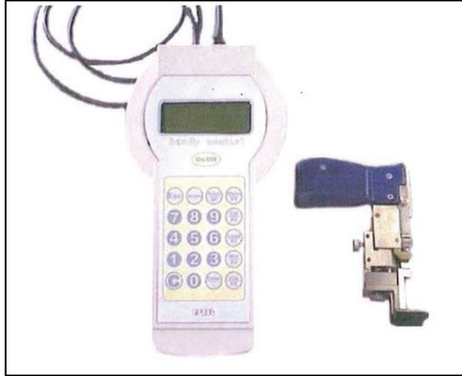
**FIGURE 3.** Image of the Ernst Handy Esatest. Provided by ApplusRTD Norway.
