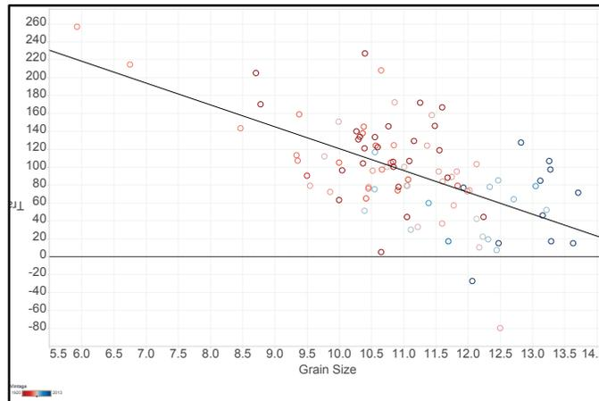
FIGURE 8. Grain size (ASTM) versus transition temperature (°F).
