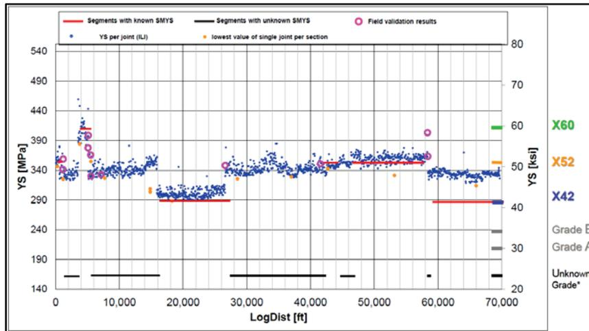
FIGURE 2. Results of the data evaluation for pipe grade determination using Rosen ILI technology. [14]
