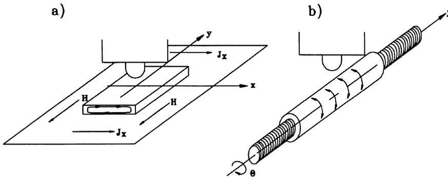
Figure 2. A schematic illustration of the inducers. (a) Parallel plate inducer, (b) Long solenoid inducer.
