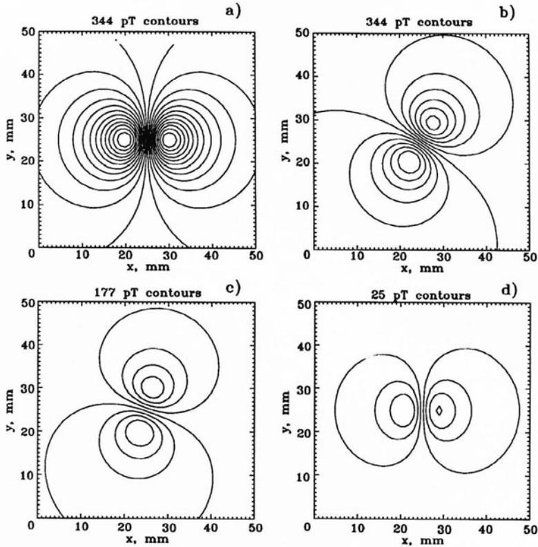
Figure 1. The calculated magnetic field map for a slot with an angle of (a)  $90^\circ$ , (b)  $30^\circ$ , (c)  $10^\circ$ , (d)  $0^\circ$  with respect to the uniform injected current. The slot is 12 mm long by 0.2 mm wide. The injected current density of  $20 \text{ A/m}^2$  is in the  $y$  direction.
