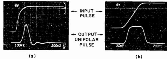
Fig. 9. The unipolar pulse generated by a commercial Panametrics 5 MHz transducer and received on an identical transducer with a high impedance electrical load. (A) Rise time of input pulse  $\approx 100$  nS (transit time in transducer); (B) Rise time of input pulse  $\gg 100$  nS.
