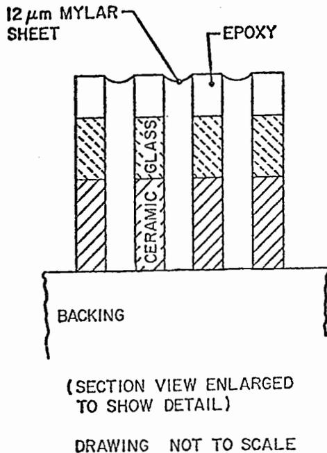
Fig. 4. Assembly drawing of longitudinal wave transducer array.
