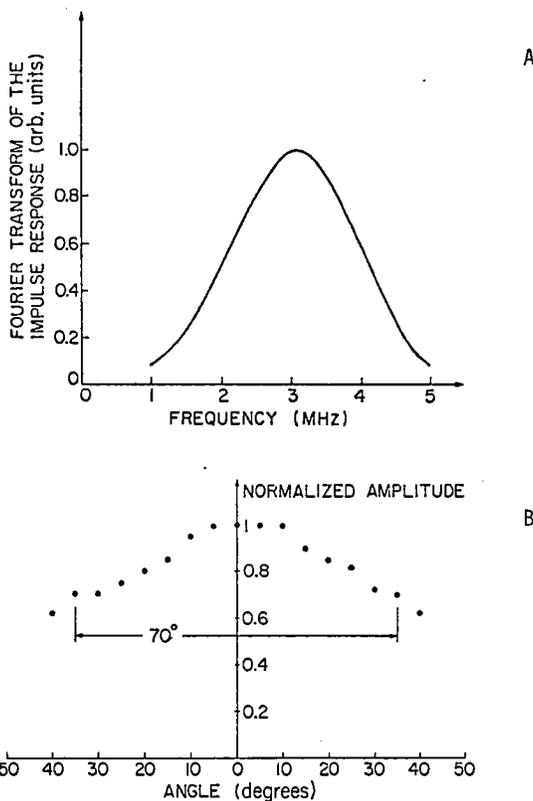
Fig. 8. (A) The impulse response and its Fourier transform of 22 elements of the array, excited in parallel, 0.5  $\mu\text{sec}/\text{Div}$  for the response; (B) the angular response of a single transducer element.
