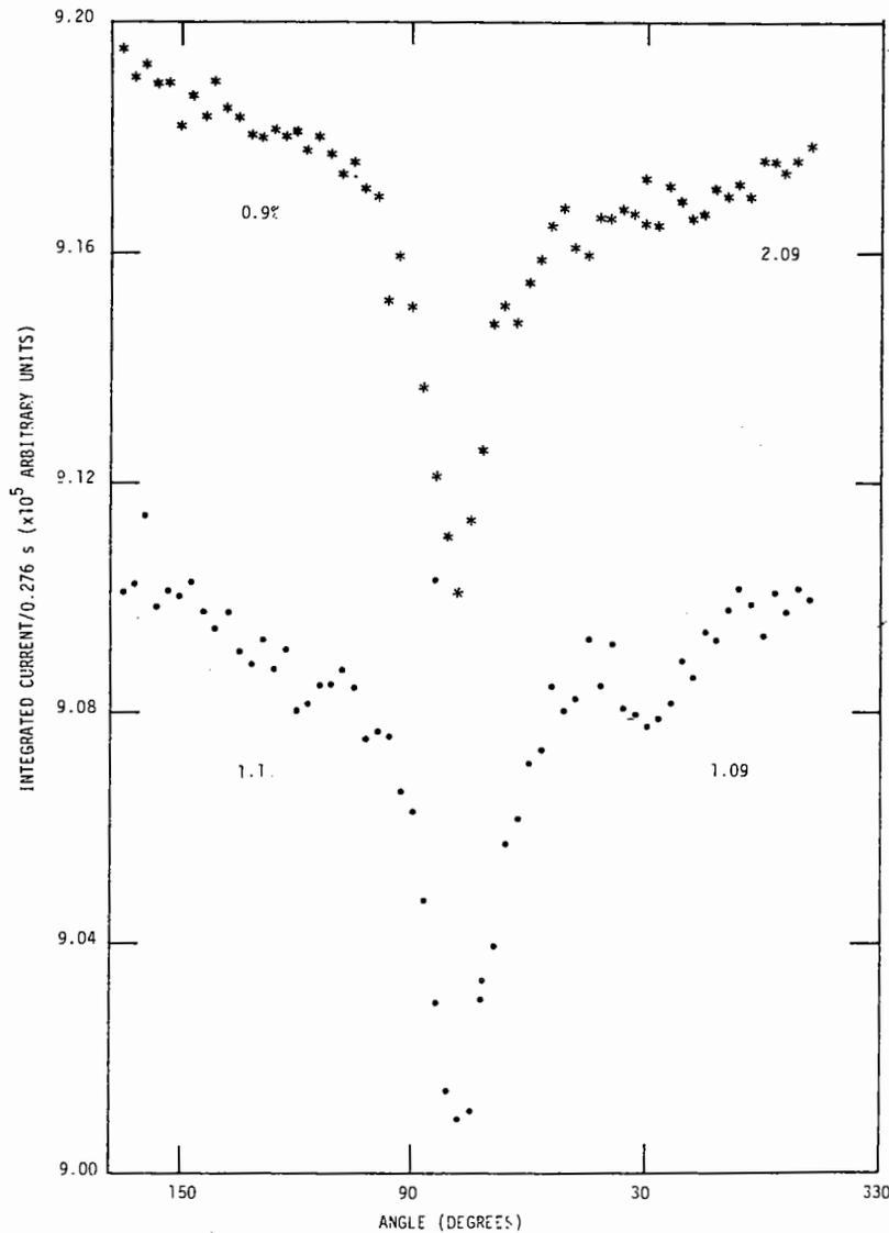
Fig. 5. Response Functions for 1/16 inch Diameter Defects 0.180 and 0.200 inch in Length at Different Distances from the Bottom of the Plastic Charge
