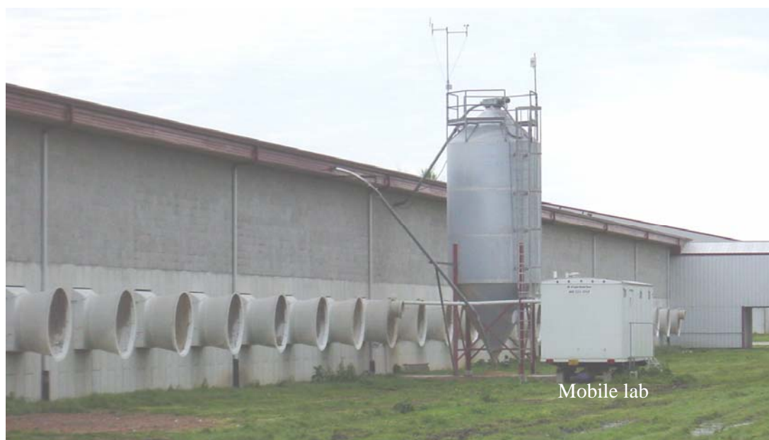
Figure 14. The Purdue University mobile lab for emission measurement installed at a laying hen facility where side-by-side comparison between the ISU portable dual-gas monitoring unit and the chemiluminescence analyzer of the mobile lab is made.
