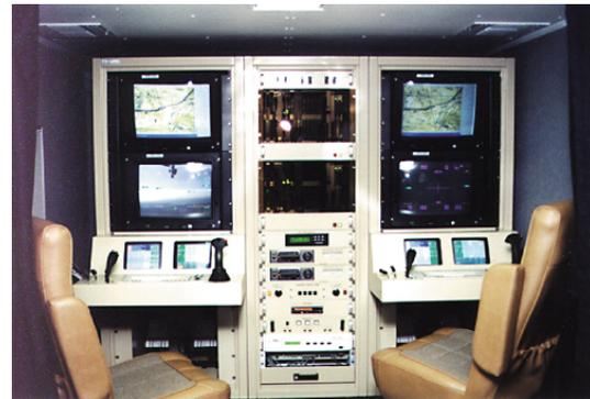
**Figure 1. Predator ground control station**
