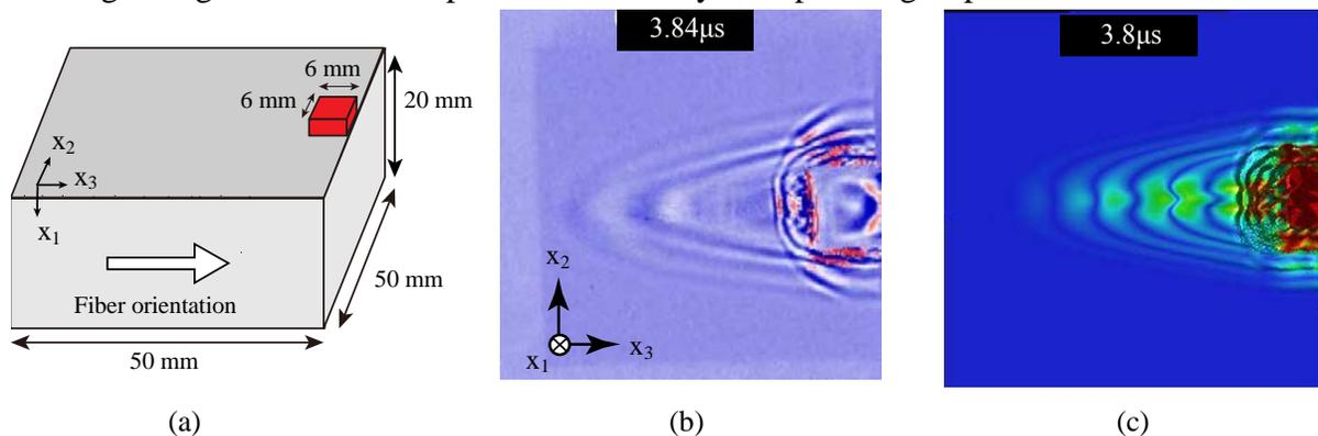
**Figure 1.** (a) CFRP specimen and location of contact transducer (1MHz), (b) visualization of wave propagation with laser scanning device, (c) result with finite element simulation.
