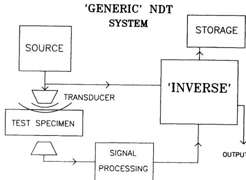
Fig. 1: The components of an NDT system.
