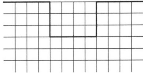
Fig. 6a: Leakage field signal for a defect in Figure 6b.
