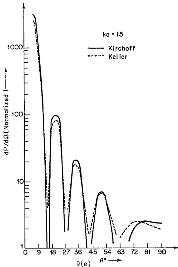
Figure 9. Scattered longitudinal power by stress free circular crack of radius  $a$ ; incident longitudinal wave along axis of crack.
