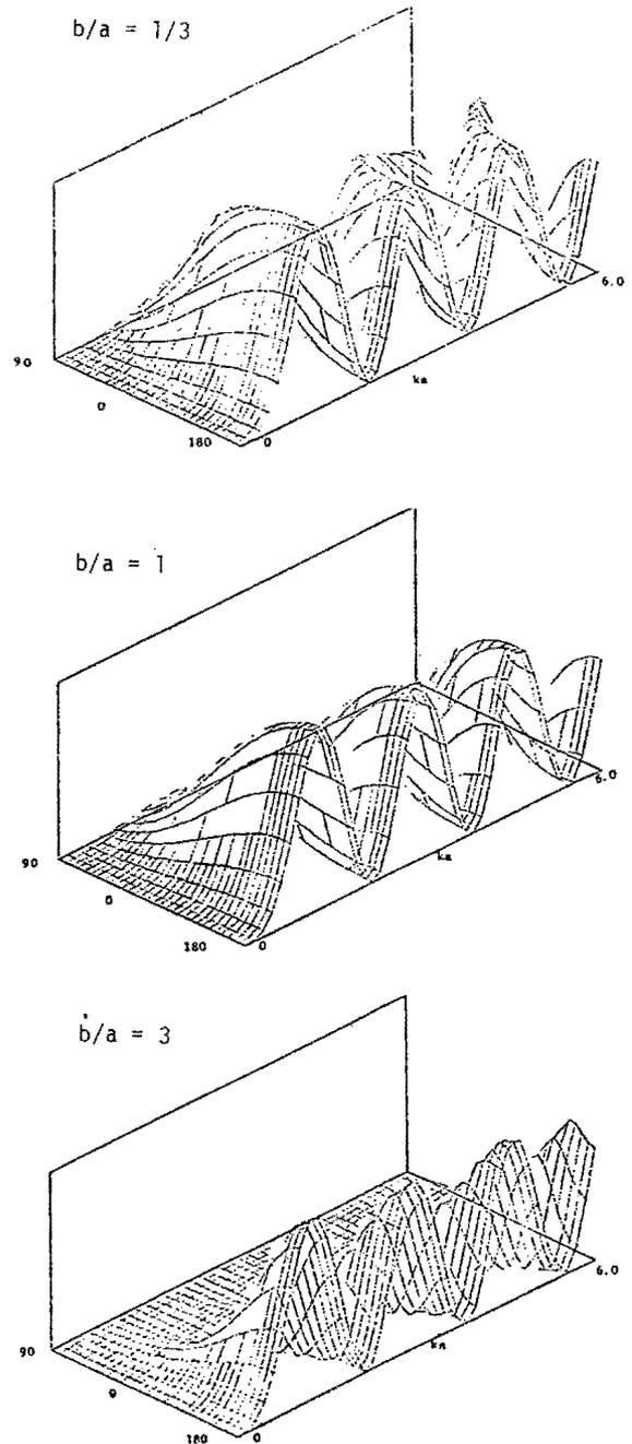
Figure 2a. Scattered (longitudinal) power for longitudinal wave incident along the symmetry axis of spheroidal scatterers (Al in Ti) of varying  $b/a$  ratio.
