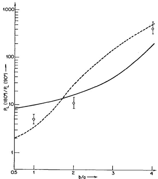
Figure 4. The ratio  $p(180/p(90))$  for longitudinal power with longitudinal wave incident along symmetry axis of spheroidal cavities in Ti, vs  $b/a$  of the scatterer. Uniform averages of  $0 < ka < 1$  (full lines) and  $0 < ka < 2$  (broken lines) were used. The circles are experimental results.
