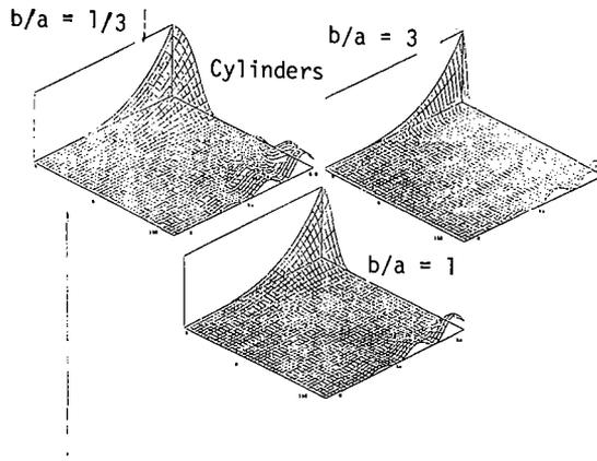
Figure 2b.. Scattered (longitudinal) power for longitudinal wave incident along the symmetry axis of cylindrical scatterers (Al in Ti) of varying b/a ratio.
