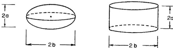
Figure 1. Cylindrical and spheroidal scatterers, characterized by  $b/a$  ratio.
