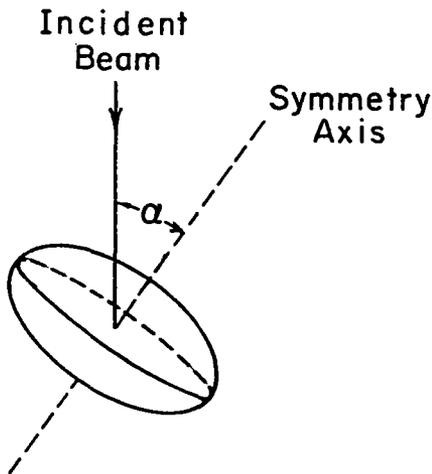
Figure 5. Scattering situation with incident beam at angle  $\alpha$  off symmetry axis of scatterer.
