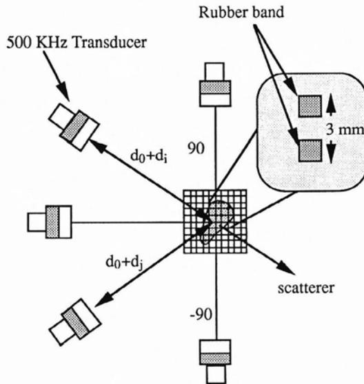
Figure 2. Diagram showing the set-up for the experiment (in actual experiment one transducer was used at different positions).
