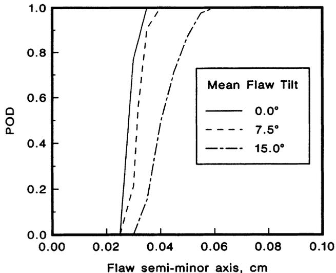
Fig. 1. Simulated POD curves for several mean flaw orientations. Angles are expressed relative to the UT beam axis (30 degree L-wave).
