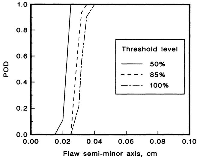
Fig. 3. Variation in POD for different detection thresholds for mean flaw tilt of 7.5 degrees relative to the UT beam. Threshold levels are expressed as percentages of the amplitude of a #1 FBH normal to the beam.
