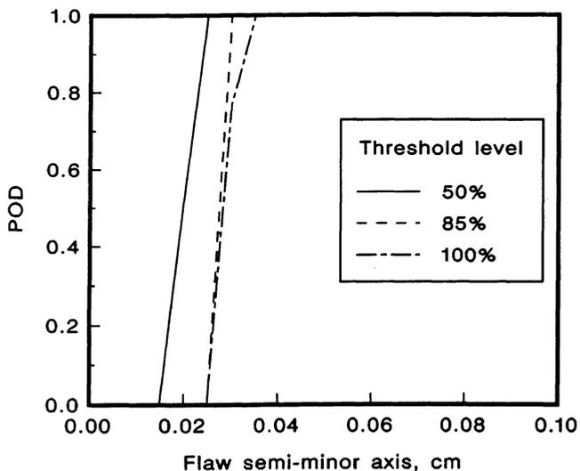
Fig. 2. Variation in POD for different detection thresholds for mean flaw orientations normal to the UT beam. Threshold levels are expressed as percentages of the amplitude of a #1 FBH normal to the beam.
