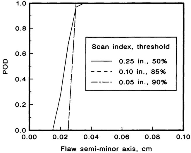
Fig. 4. Variation of POD of defects with mean orientations normal to the UT beam for different scan index values. Thresholds are expressed as a percentage of the amplitude of a #1 FBH normal to the beam.
