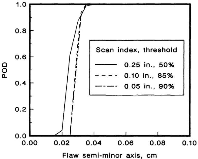
Fig. 5. Variation of POD of defects with a mean tilt of 7.5 degrees relative to the UT beam for different scan index values. Thresholds are expressed as a percentage of the amplitude of a #1 FBH normal to the UT beam.
